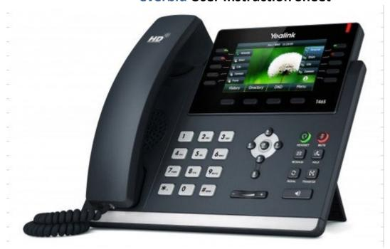
The main hardware components of the SIP-T46S IP phone are the LCD screen and the keypad.
